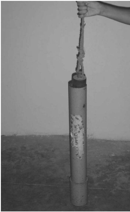
Fig. 4—Protodyakonov's apparatus for determination of compressive strength of rock samples.
