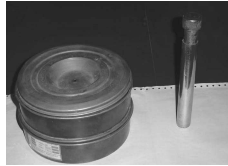
Fig. 5—Test sieve and measuring cylinder used in Protodyakonov's test.
