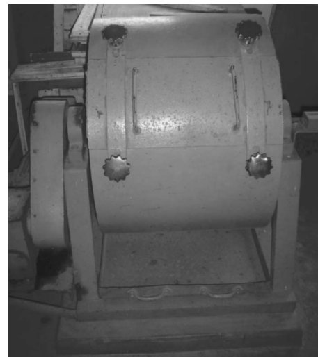
Fig. 6—Los Angeles' abrasion test apparatus for determination of abrasivity of rock samples.
