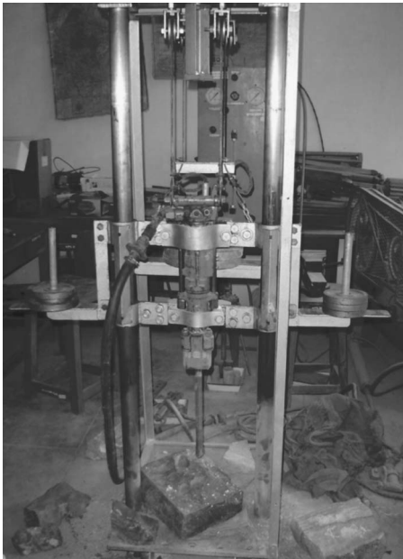
Fig. 3—Jackhammer drill setup for drilling vertical holes in rock samples.
