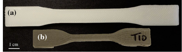
Fig. 1. 3D-printed (a) HDPE and (b) HDPE40-2X tensile bar.
