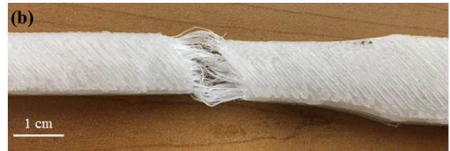
Fig. 2. (a) Representative stress–strain curve for HDPE tensile samples at strain rate of 10^{-3} \text{ s}^{-1} , and (b) failure mode for HDPE tensile bar at 50% strain.
