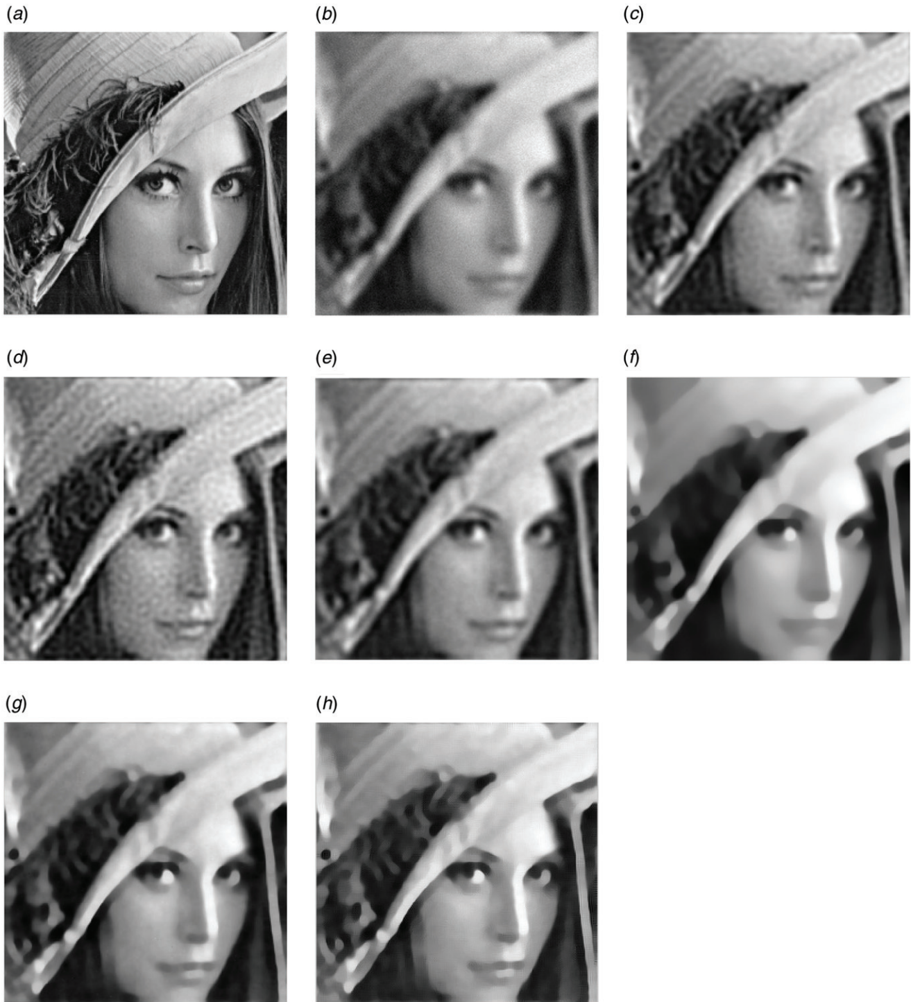
Figure 2. Results of various filters applied to the image “Lena”: (a) original figure; (b) blur and noisy figure (out of focus blur generated using a Gaussian kernel; SNR of noisy image is 10 dB); (c) after applying the FFT-REG filter; (d) after applying the SOB-REG filter; (e) after applying the Tikhonov method; (f) result of applying the TV model; (g) result of the MO model; (h) result of the proposed model. Row profile of the image “Lena” (200th row is selected): the one-dimensional profile of the original, noisy and reconstructed images: (i) after applying the FFT-REG filter; (j) after applying the SOB-REG filter; (k) after applying the Tikhonov method (l) result of applying the TV model; (m) result of the MO model; (n) result of the proposed model. (The color version of this figure is included in the online version of the journal.)
