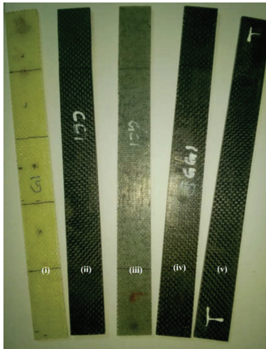
FIGURE 2. Extracted composite beams: (i) 16 layer glass and (ii) 16 layer carbon, and hybrid are (iii) GC1, (iv) GG1 and (v) CC1.
