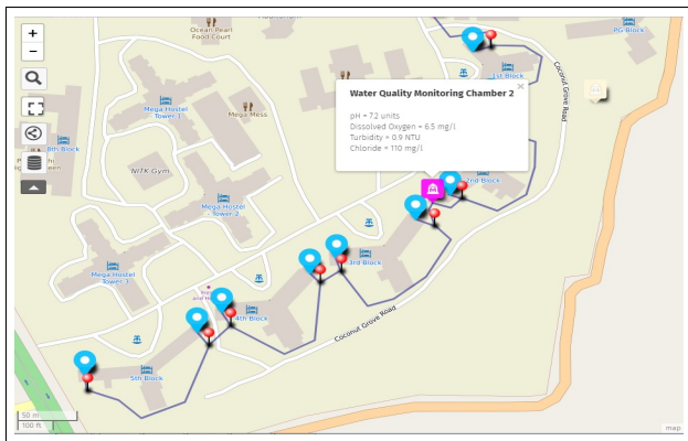
Fig. 11. Water flow and water quality display on GUI in real time map
