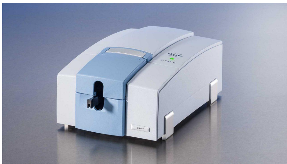
Fig. 2.6 FTIR setup (Image courtesy: Chemistry department, NITK, Surathkal)
