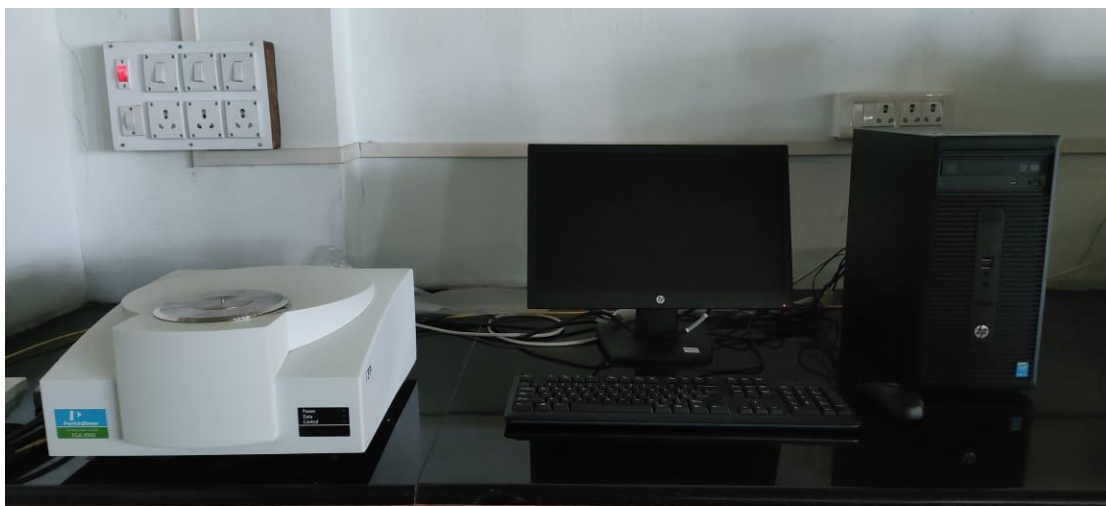
Fig. 2.7 TGA setup (Image courtesy: Chemistry department, NITK, Surathkal)
