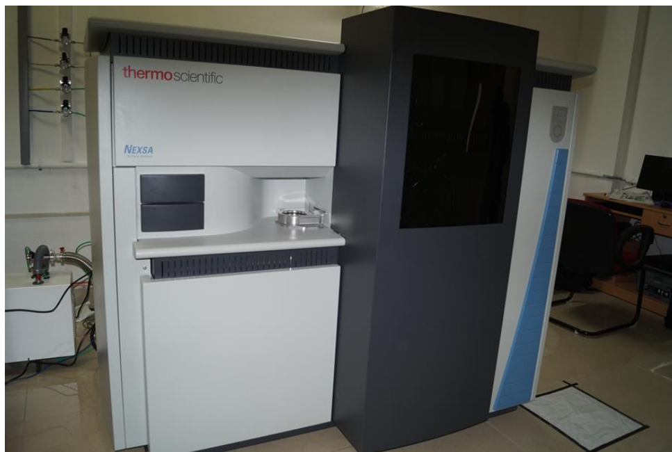
Fig. 2.11 XPS setup (Image courtesy: Advanced material research center. IIT Mandi)
