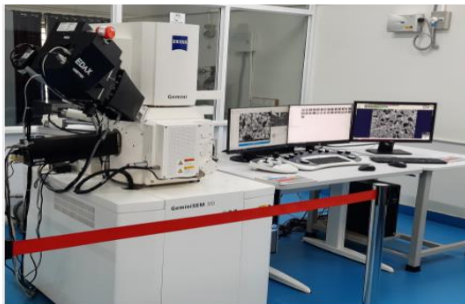
Fig. 2.9 FESEM and EDS setup (Image courtesy: Central research facility (CRF), NITK, Surathkal)
