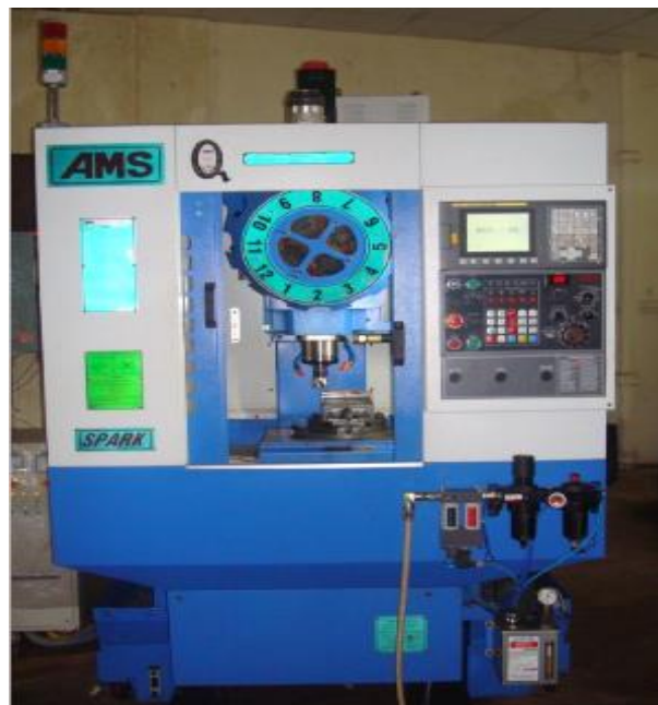
Figure 3.3(a): Experimental setup CNC vertical milling machine (Spark DTC 250)
