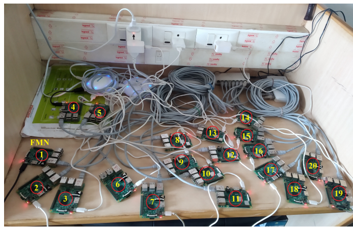
Figure 4.6: Fog Computing Testbed for performance evaluation
