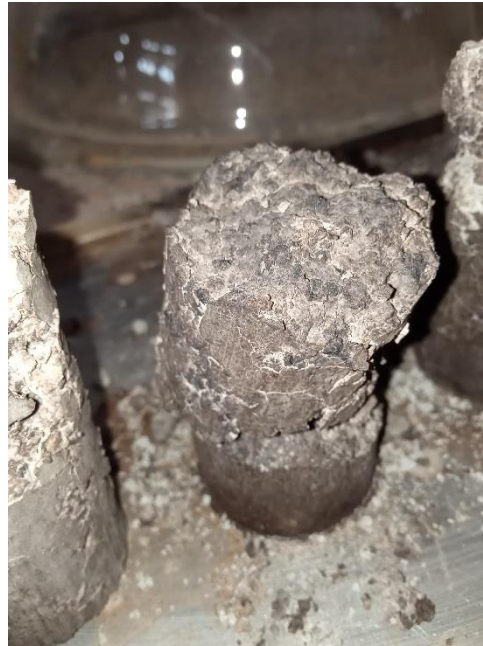
(b) Soaked specimens were bulged and exhibited deterioration during the drying cycle
