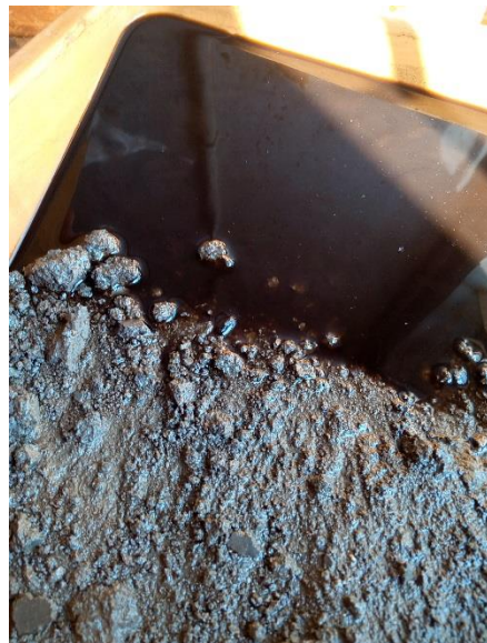
(d) Water turned into a blackish colour with the softened alkali-activated soil
