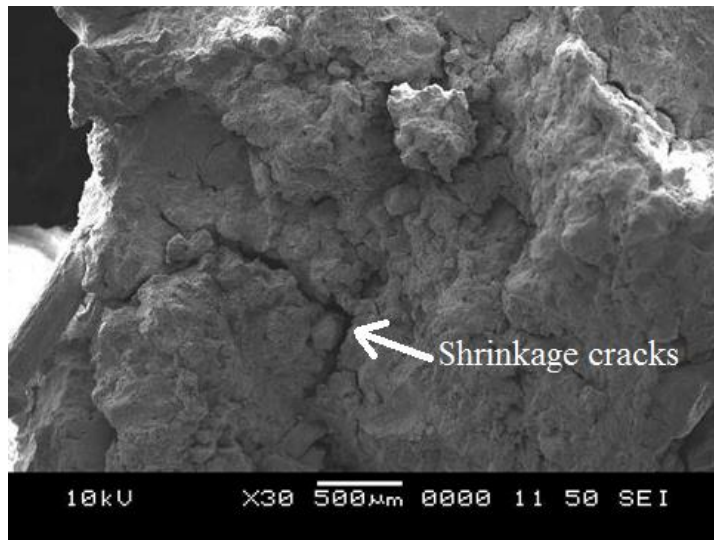
(a) Dry BC soil with shrinkage cracks
