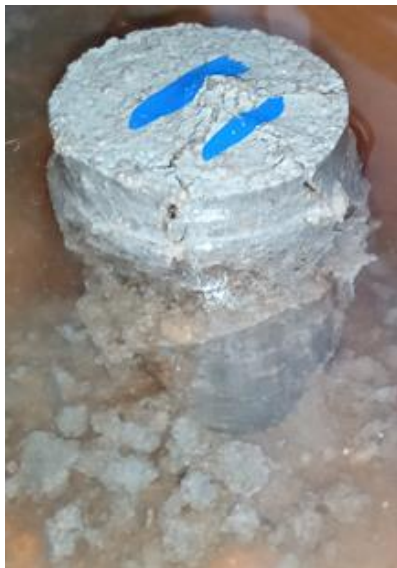
(c) Failure of alkali-activated soil with fly ash during soaking cycle
