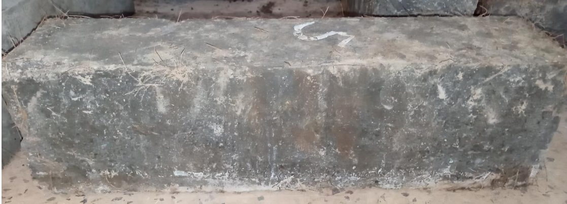
Figure 4. 22 Beam specimen of BC soil stabilized with Cement, fly ash, and 0.5% coconut fiber without cracks
