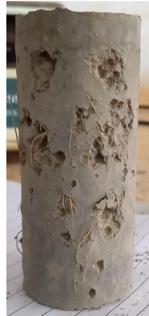
f) Cement-fly ash stabilized WD specimen with coconut fibers
