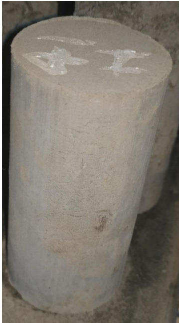
(d) Cement-fly ash stabilized soil specimen without soil loss
