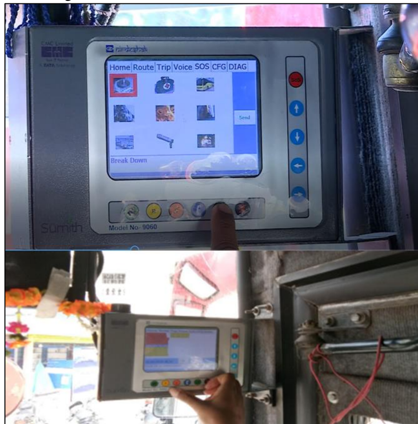
Figure 3.6 Vehicle Mounted Unit (VMU) - GPS
