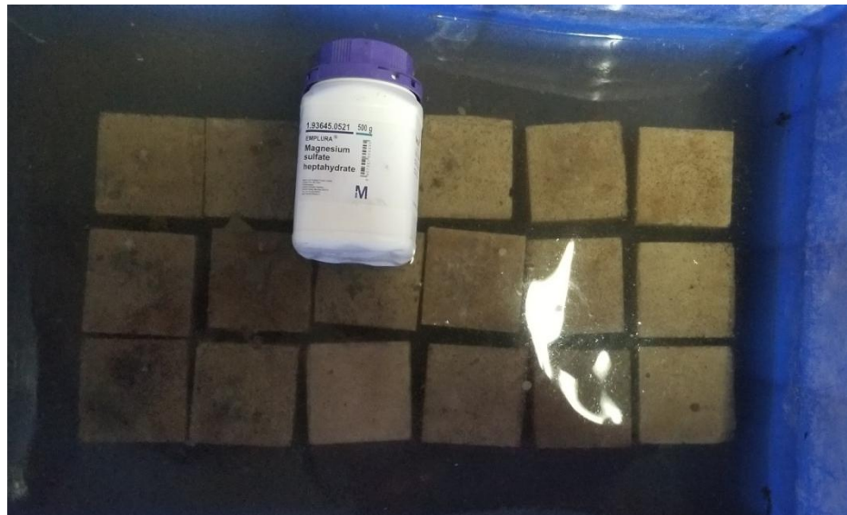
Figure 3.7: FCA based AAS mortar mixtures exposed to MgSO_4 solution.
