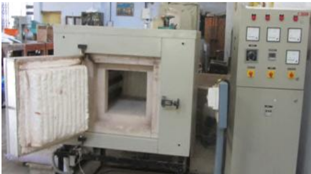
Figure 3.8: Programmable electric furnace used for elevated temperature studies.
