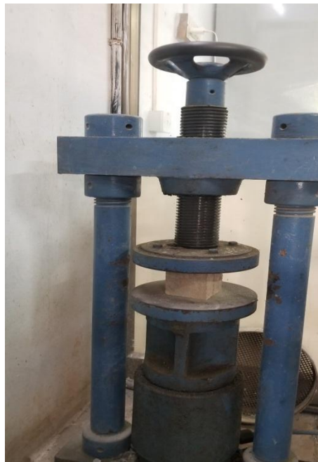
Figure 3.5: Compressive strength testing setup.
