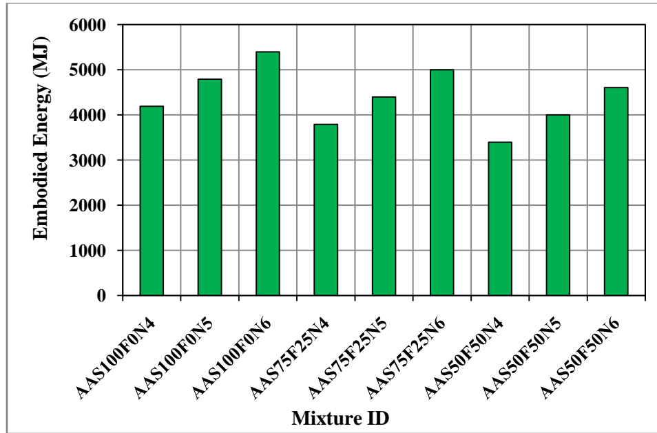
Figure 6.3: EE_{eq} values of FCA based AAS mortar mixtures for varies levels alkaline solution of concentration (i.e., 4 - 6% Na_2O dosage).
