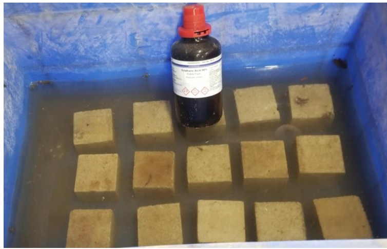
Figure 3.6: FCA based AAS mortar mixtures exposed to acid solution.
