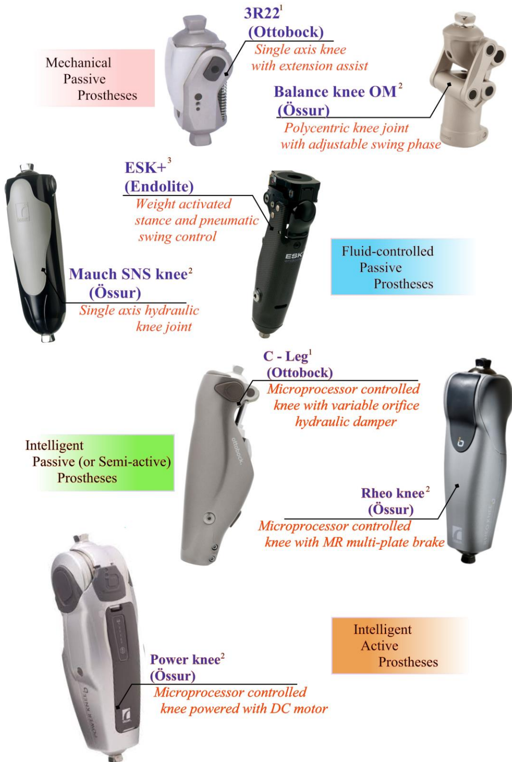
Figure 2.2 Evolution of knee prostheses (Source: 1 www.ottobock.com, 2 www.ossur.com, 3 www.blatchfordus.com)
