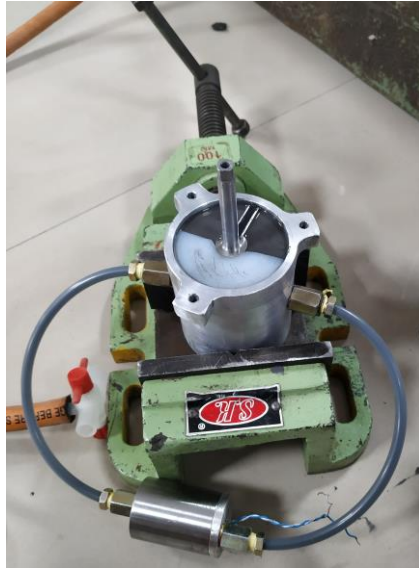
Figure 6.10 Rotary chamber filled with MR fluid
