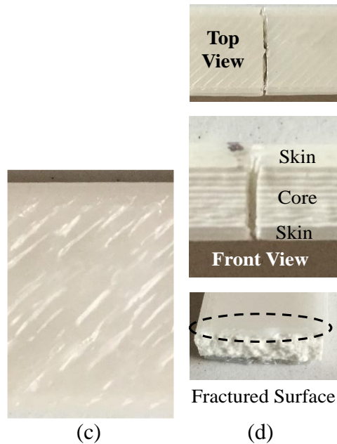
Figure 5.12 Schematic representation of (a) core indentation and (b) failure modes observed in 3D printed SF core sandwiches (c) face wrinkling in SH20 and (d) indentation failure (SH40 and SH60).
