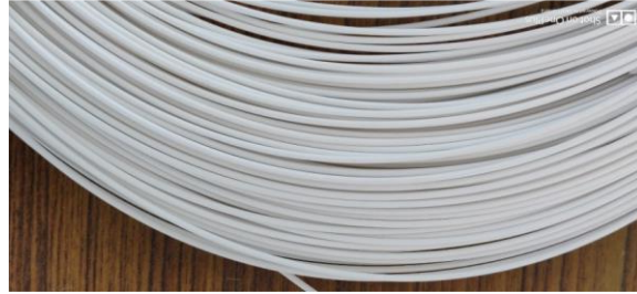
Figure 3.3 Representative extruded H60 feedstock filament.
