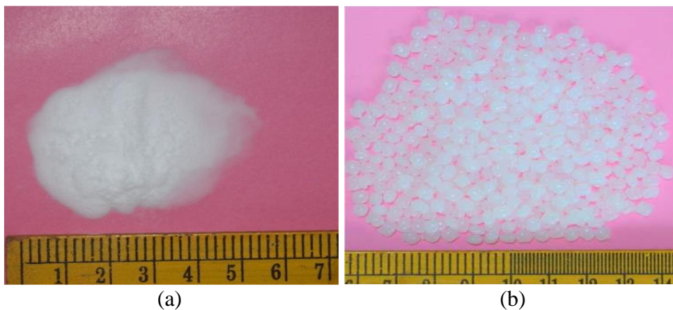
Figure 2.1 As received (a) GMB in powder form and (b) HDPE granules used in the present work.
