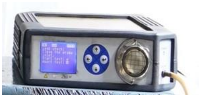
Plate 3.10 Measurement Panel of AVL exhaust gas analyzer
