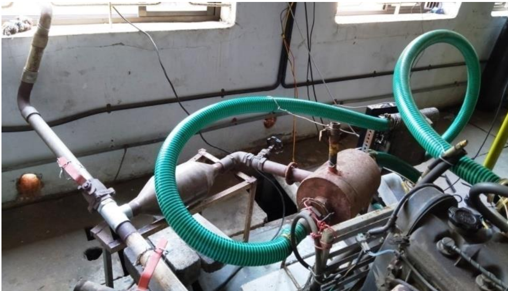
Plate 3.7 Fabrication for part cooled exhaust gas recirculation
