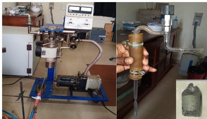
Figure 2.5: (a) Evacuation unit. (b) Quartz ampoule (Inset shows the image of the ingot).
