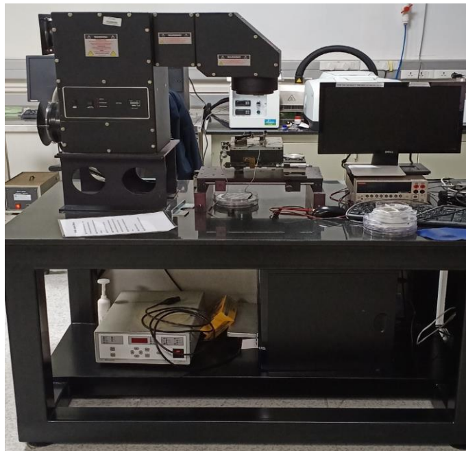
Figure 2.27: Newport Sol3A class AAA solar simulator.
