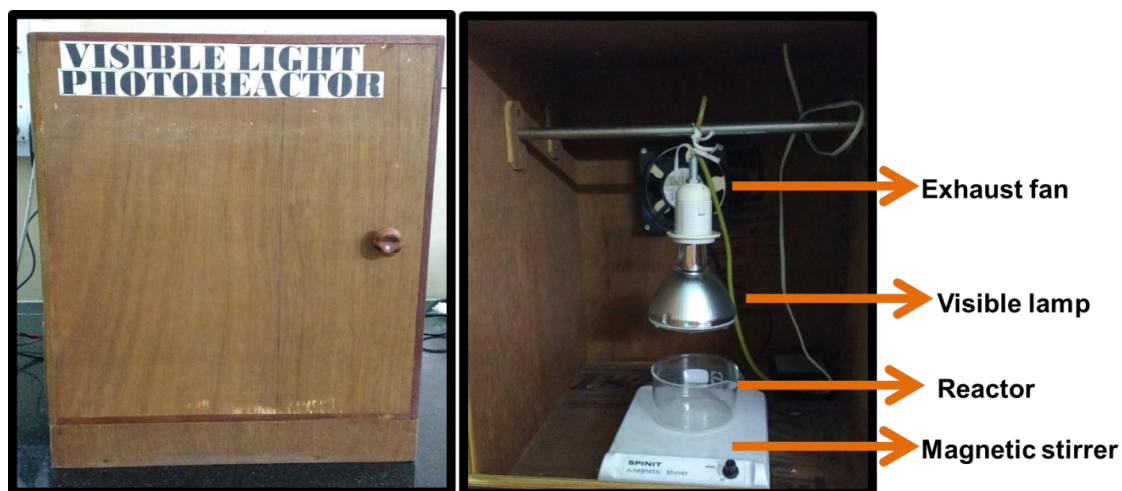
Figure 2.2: Color photograph showing the different components of the home-made visible light photoreactor
