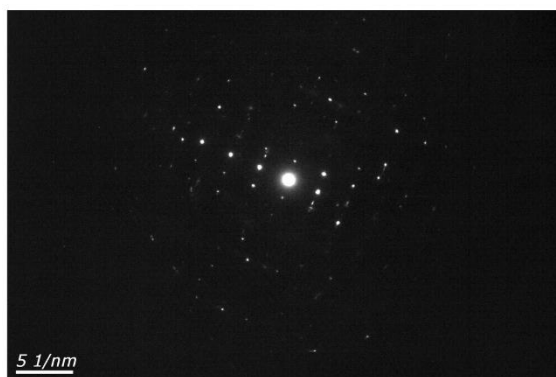
Figure 3.11: Selected area electron diffraction (SAED) pattern of 3D CdS obtained through transmission electron microscopy.
