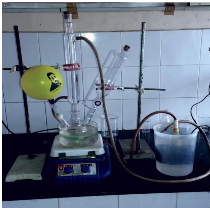
Fig. 3.1 Set-up for the synthesis of Ag and Ag-Cu alloy nanoparticles by poly-ol method.
