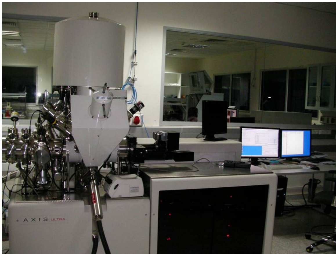
Figure 3.12: Multi-technique X-ray Photoelectron Spectroscopy with XPS-mapping capability
