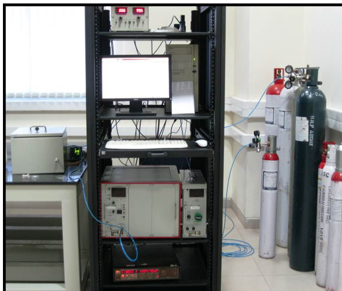
Figure 3.16: Gas sensor setup used for O 2 sensitivity measurement
