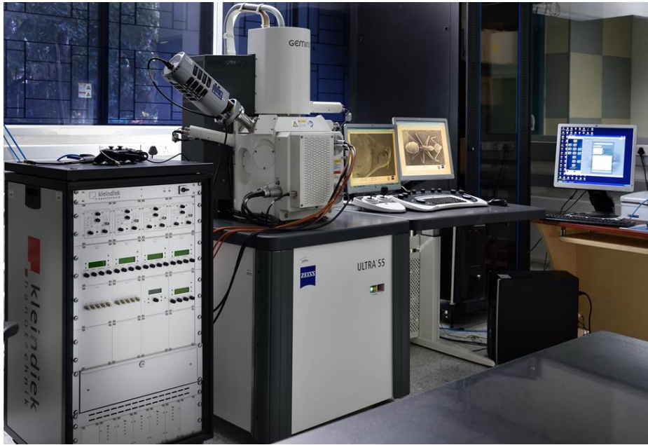
Figure 3.9: ULTRA 55 - Ultra high resolution scanning electron imaging coupled with material spectroscopy tools
