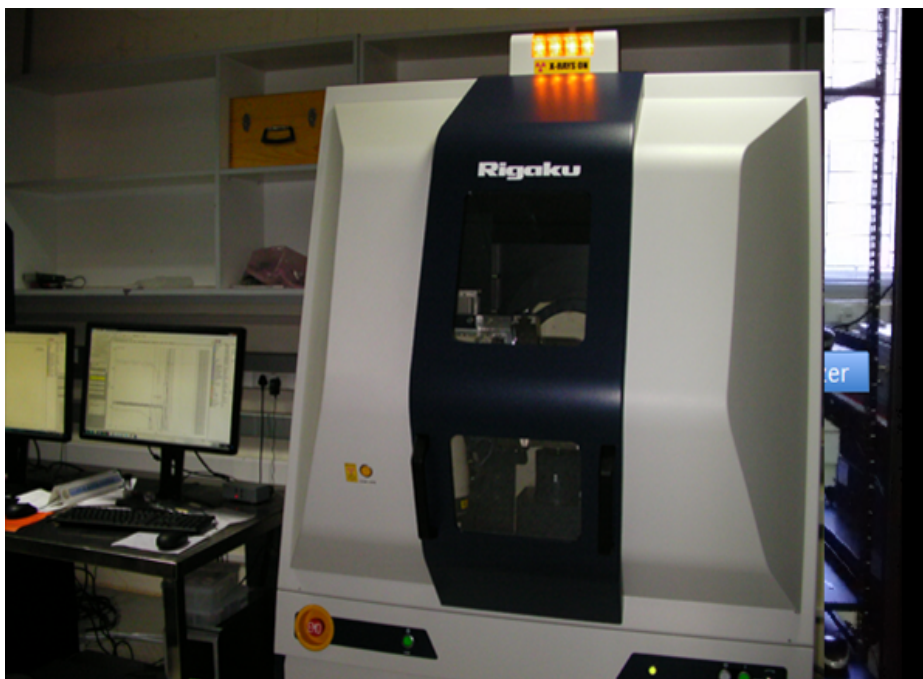
Figure 3.11: Rigaku SmartLab High Resolution X-ray Diffractometer system.
