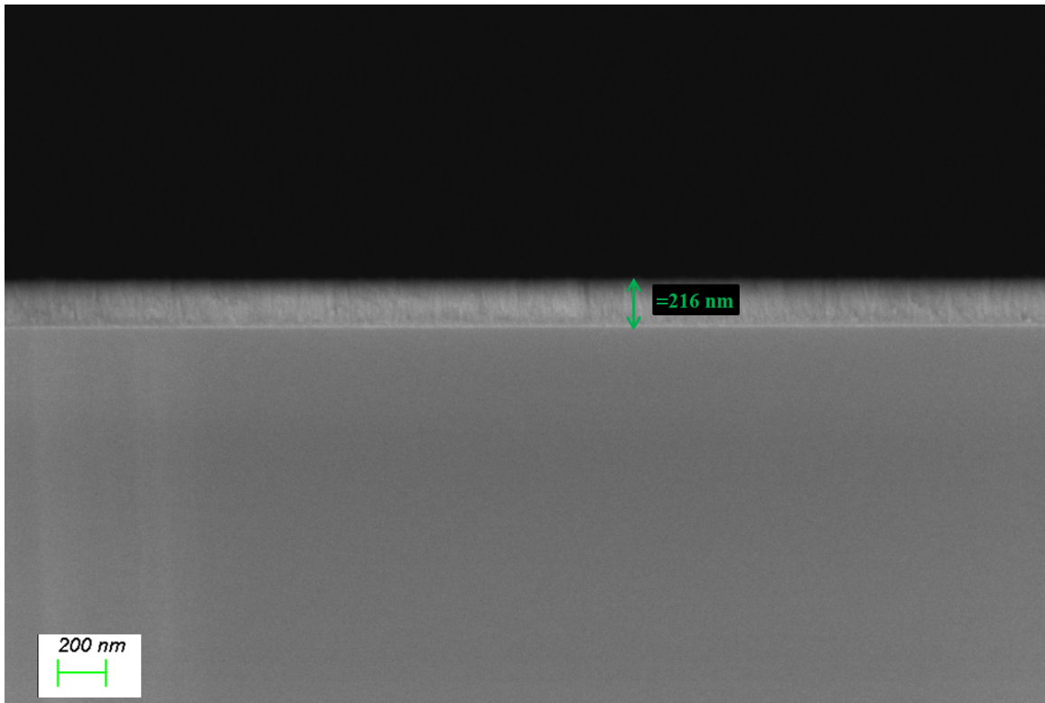
Figure 5.1: Cross-sectional SEM image of the \text{CeO}_2\text{-HfO}_2 film deposited for 180 minutes
