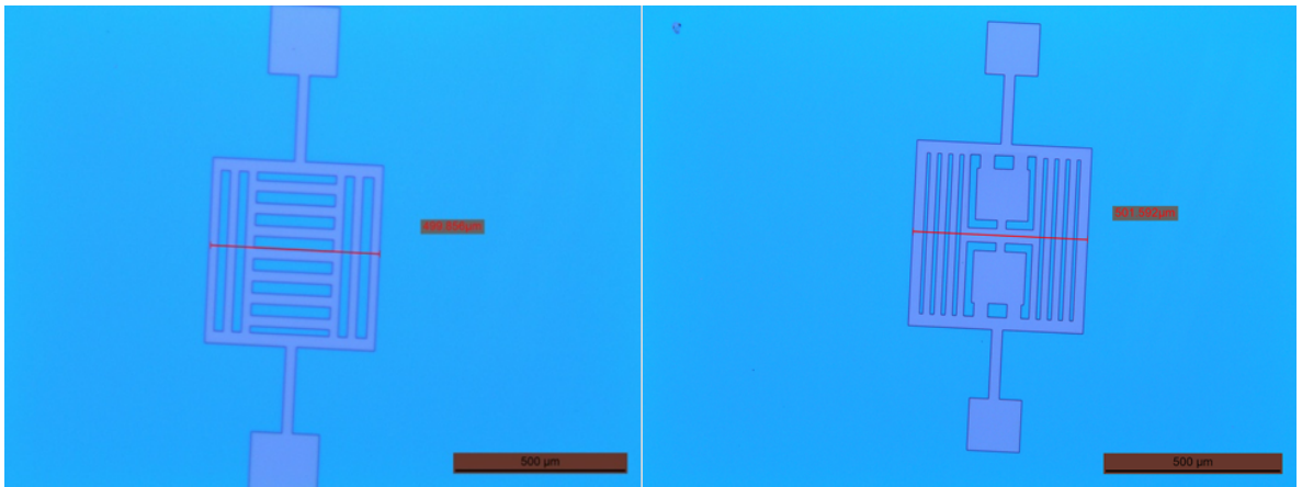
Figure 6.8: Visual inspection of fabricated microheaters using optical microscope.
