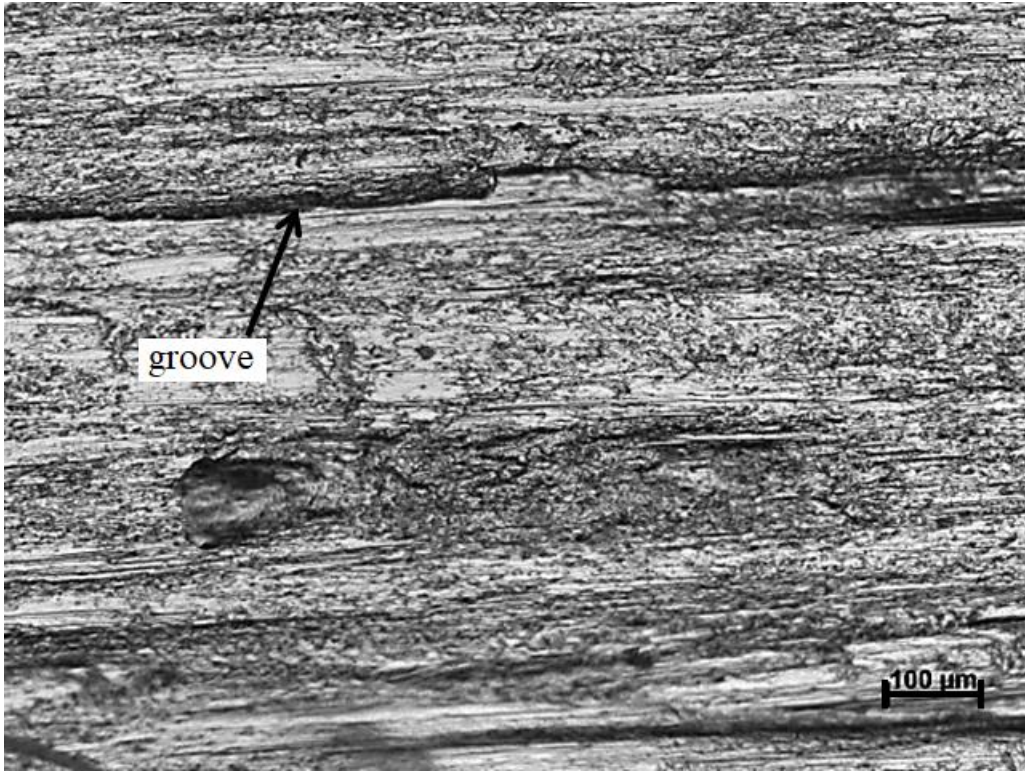
Figure 5.38: Micrograph of worn disk specimen tested at 2 kg normal load, 2 m/s sliding speed and at room temperature.
