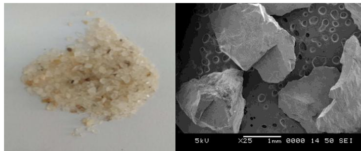
Figure 3.24 Sand used as abrasive medium
