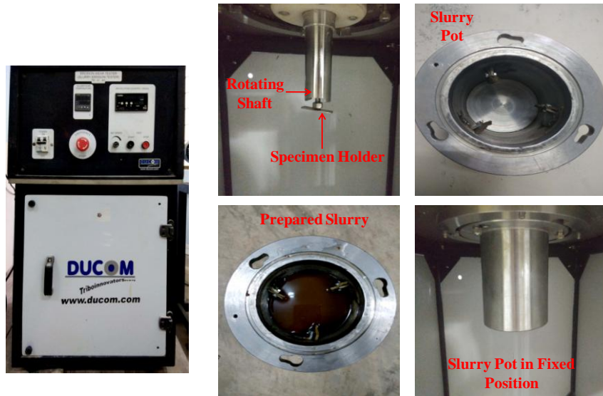
Figure 3.23 Slurry erosion setup
