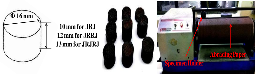
Figure 3.25 Samples, schematic and DIN abrader
