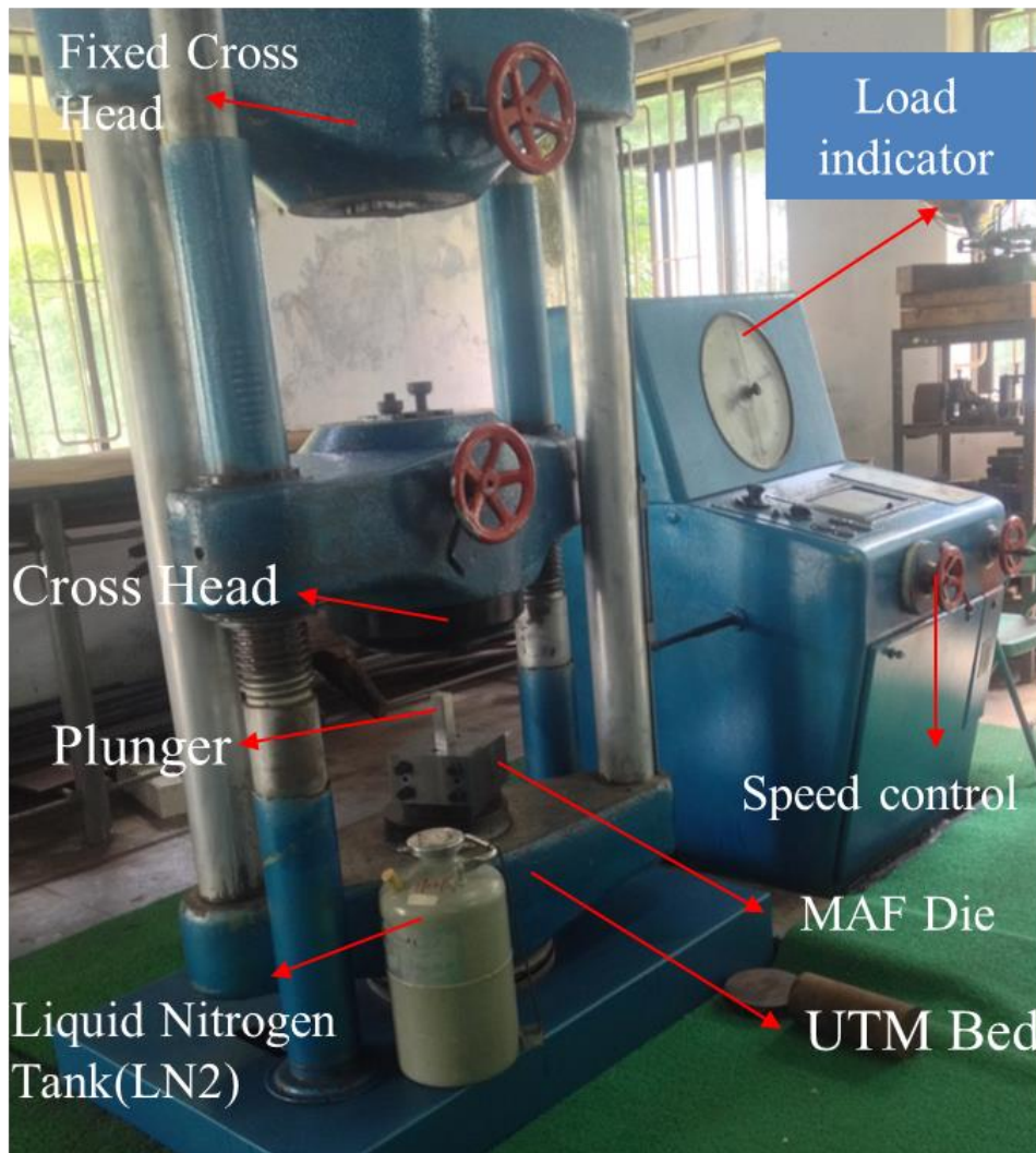
Figure 3.2 Universal Testing Machine used in the experimental process.
