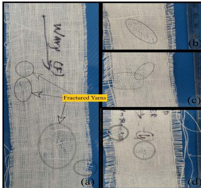
Figure 5.3: The fractured fabrics after tensile test, (a) P1, (b) Magnified fracture area of P2, (c) Magnified fracture area of P2, and (d) Magnified fracture area of WR.
