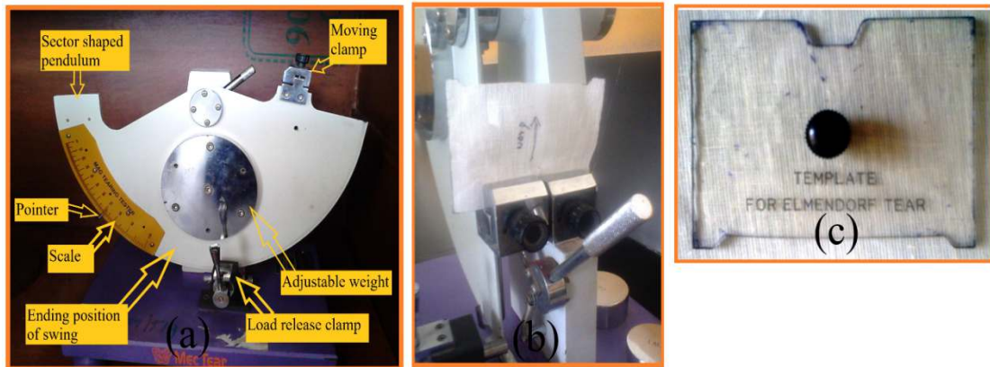
Figure 3.5: Impact tearing tester (a) Elmendorf tear tester (b) Fabric mounted by fixing both the ends of fabric (c) Tearing testing template which is placed on P1 types of sisal fabric
