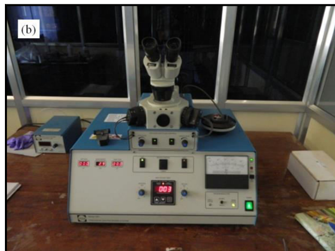
Fig. 3.5 a) Transmission electron microscope JEOL-JEM 2100, b) PIPS ion milling unit
