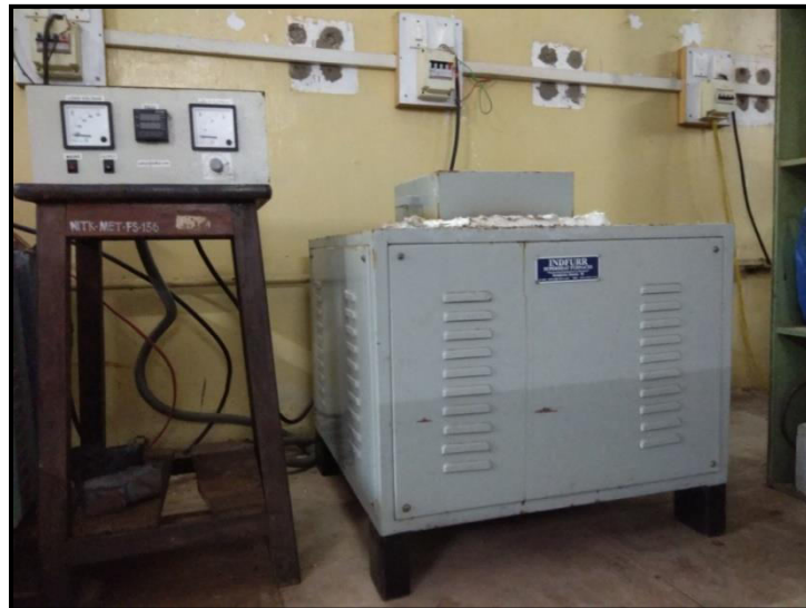
Fig. 3.3 Salt bath furnace used to carry out heat treatment
