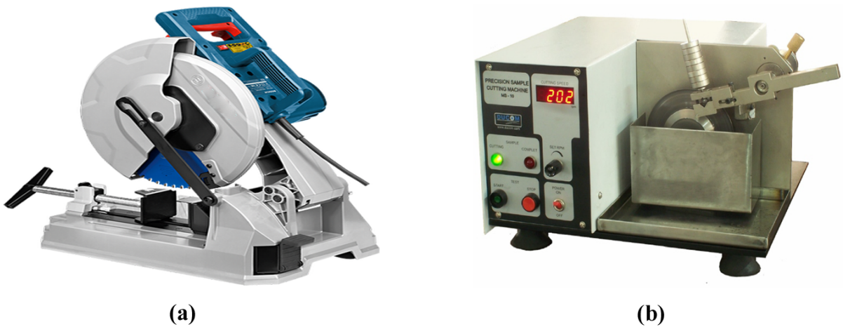
Figure 3.4: Two types of cutters used for cutting the cored reinforced concrete samples, (a) high speed diamond saw cutter and (b) low-speed precision diamond saw cutter
