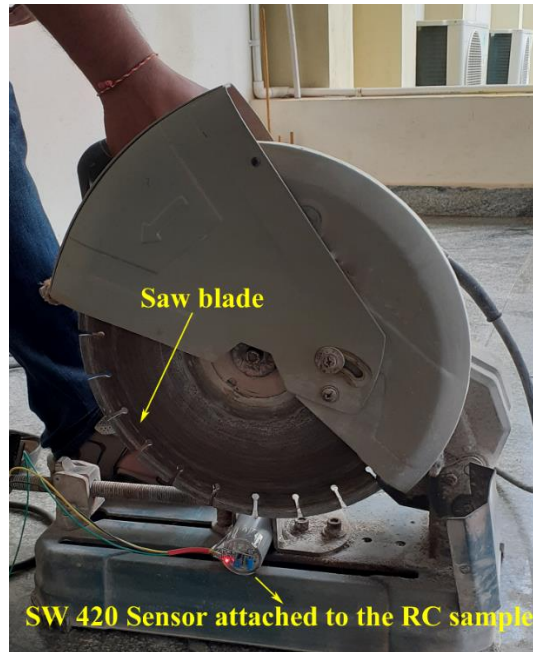
Figure 3.8: Sample cutting while vibration sensor (SW 420) attached to the RC sample
