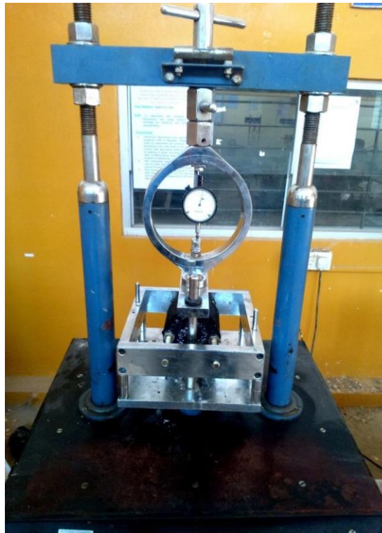
Figure 3.9 Indirect Tensile Strength Test set up
