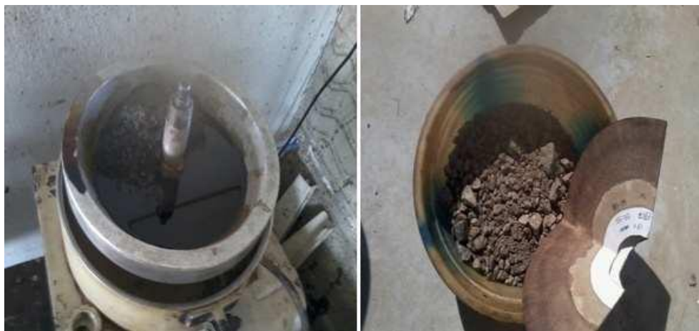
Figure 3.4 Binder recovery through Centrifuge Extractor.
