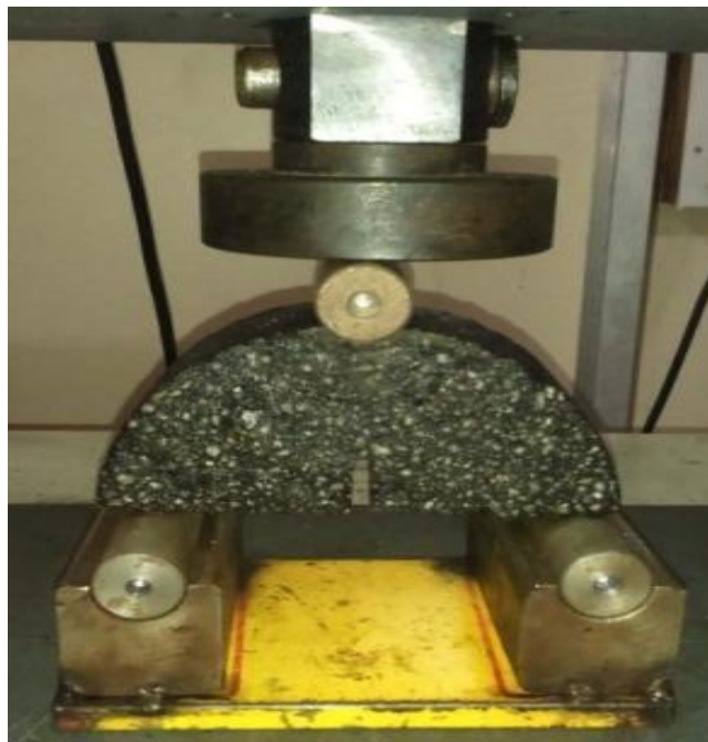
Figure 3.14 Semi Circular Bending test on sample
