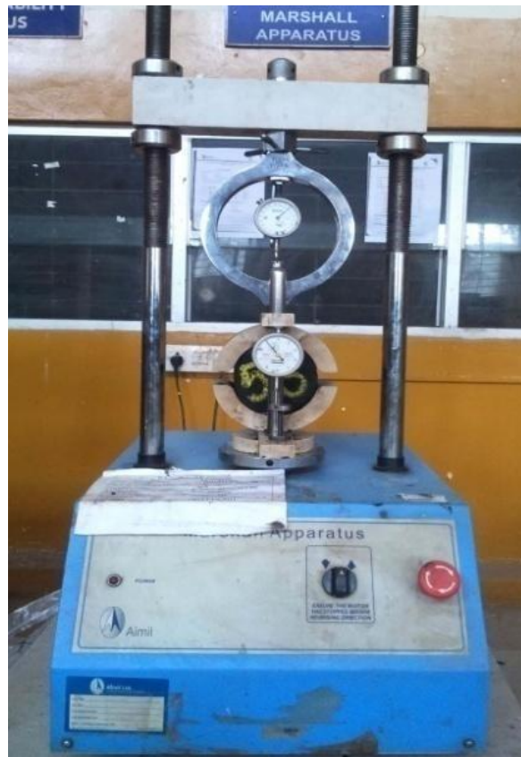
Fig. 3.8 Marshall Test Setup
