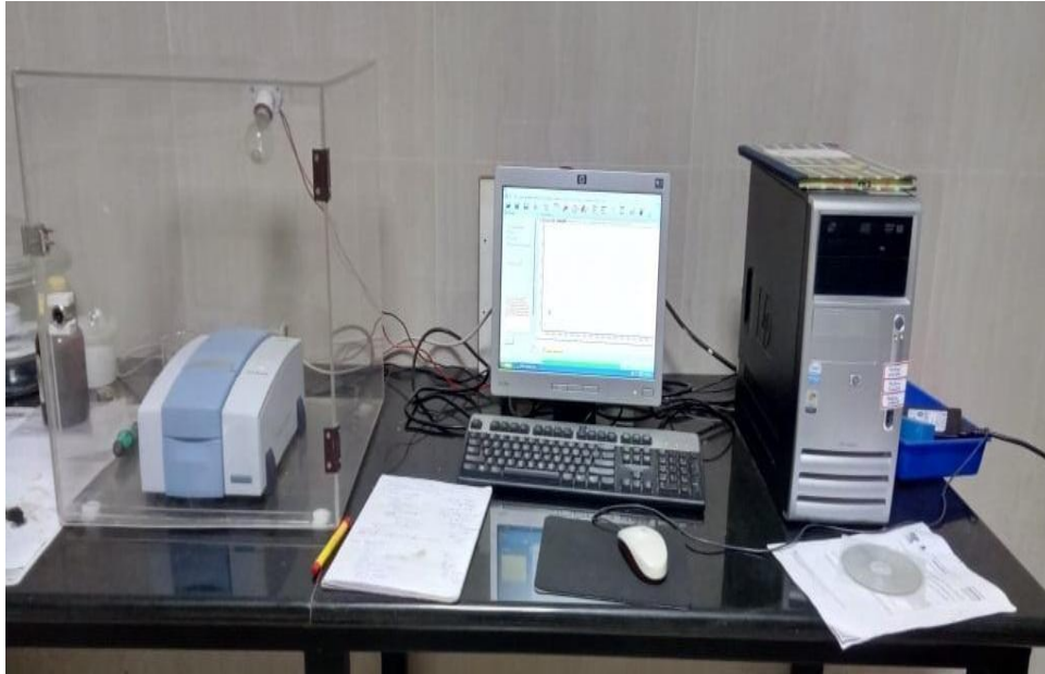
Figure 3.7 Fourier Transform Infrared Spectroscopy set up
