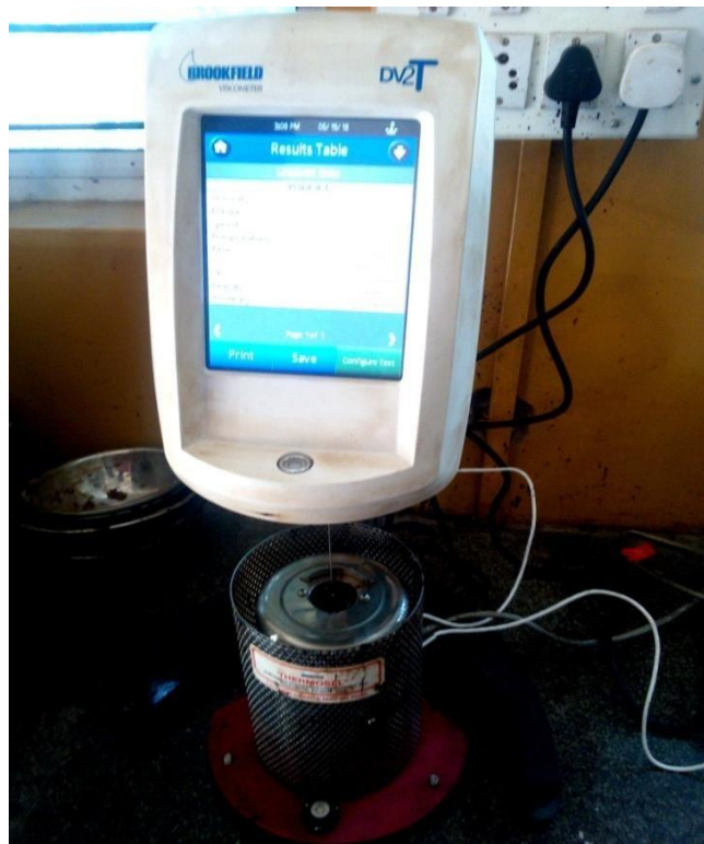
Figure 3.5 Brookfield Rotational Viscometer The test temperature of 135 0 C (kinematic viscosity) was maintained
