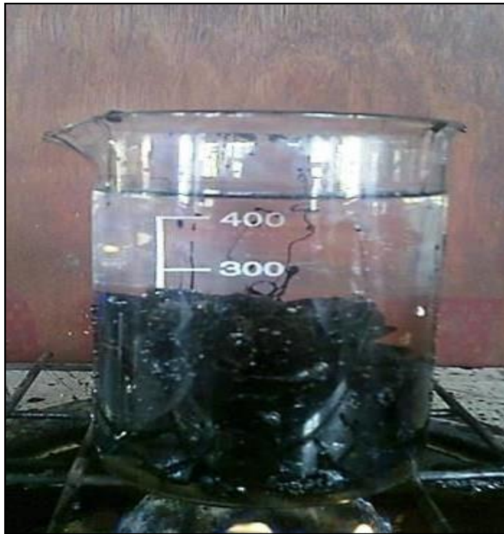
Figure 3.13 Sample of SMA mix for Boiling Test
