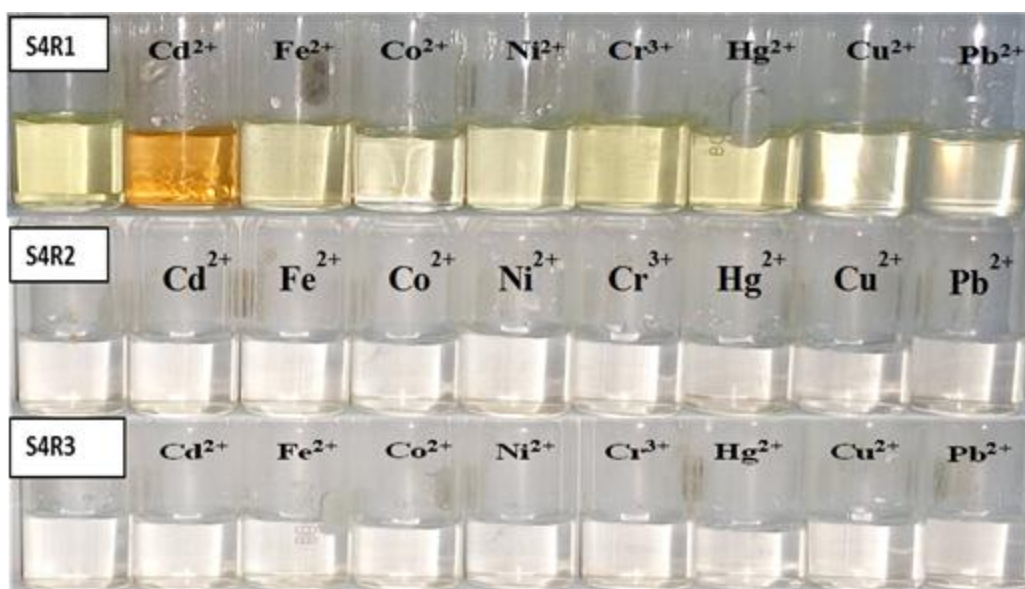
Fig. 5.13. The colorimetric changes of receptor S4R1–S4R3 upon addition of 2.0 equiv. of various cations in an aqueous solution
