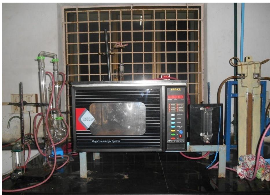
Fig. 3.2. Pictorial representation of the microwave reactor
