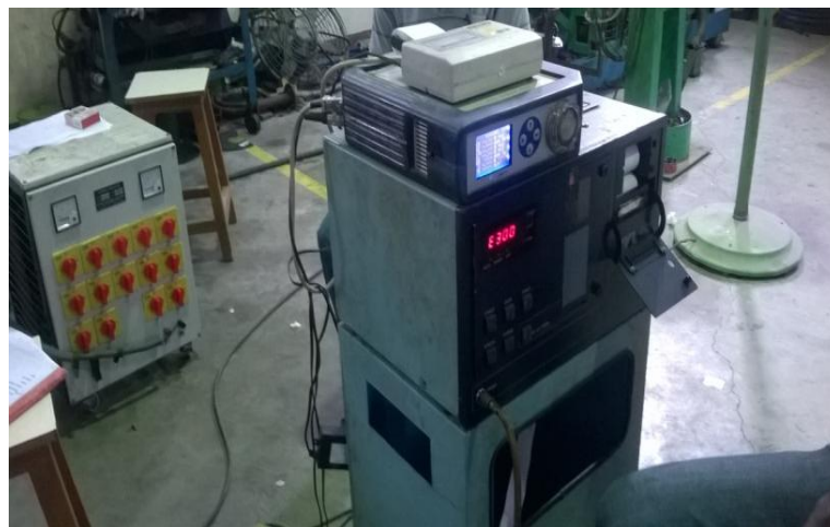
Fig 4.3 Five Gas analyser and smoke meter.
