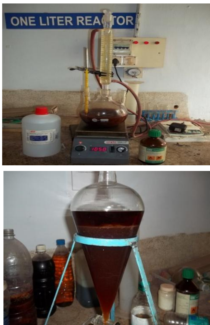
Fig 5.7 Acid Esterification and acid Layer separation
