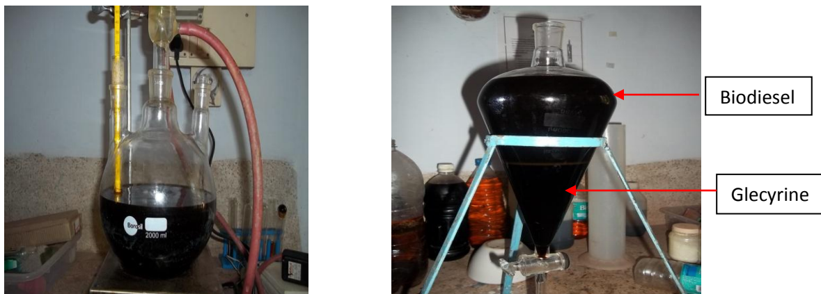
Fig 5.8 Base esterification and Biodiesel separation
