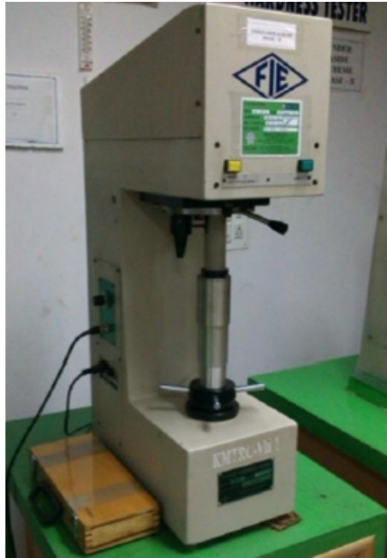
Figure 3.9 Vickers hardness testing machine.
