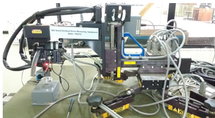
Figure 3.13 Residual stress testing machine.
