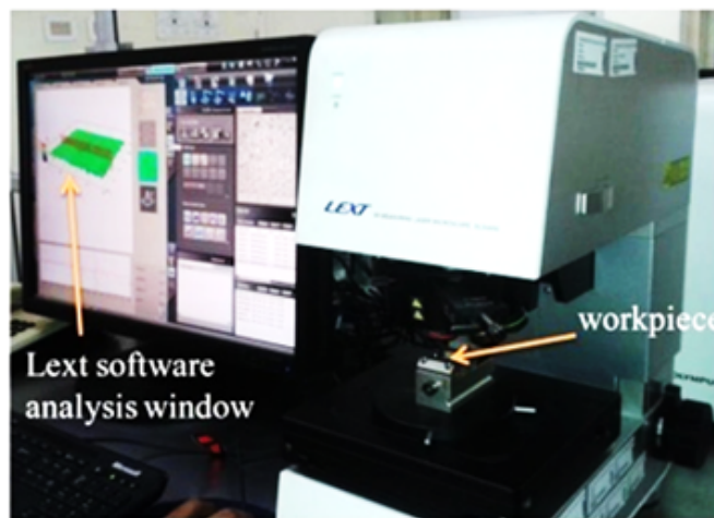
Figure 3.11 Laser optical confocal microscope.
