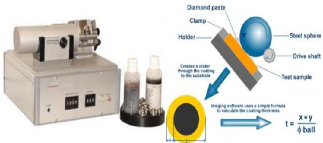
Figure 3.18 Calo tester used for coating thickness measurement (Courtesy: Oerlikon Balzers Pvt. Ltd., India).
