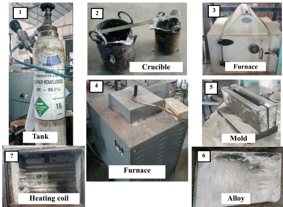
Figure 3.1 Magnesium casting facility (Courtesy: CSIR-NIIST)
