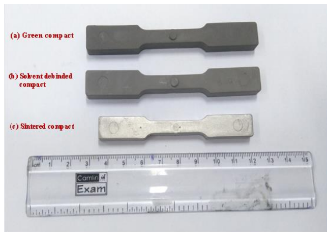
Figure 3.26 Tensile specimen sintered at 1200 °C
