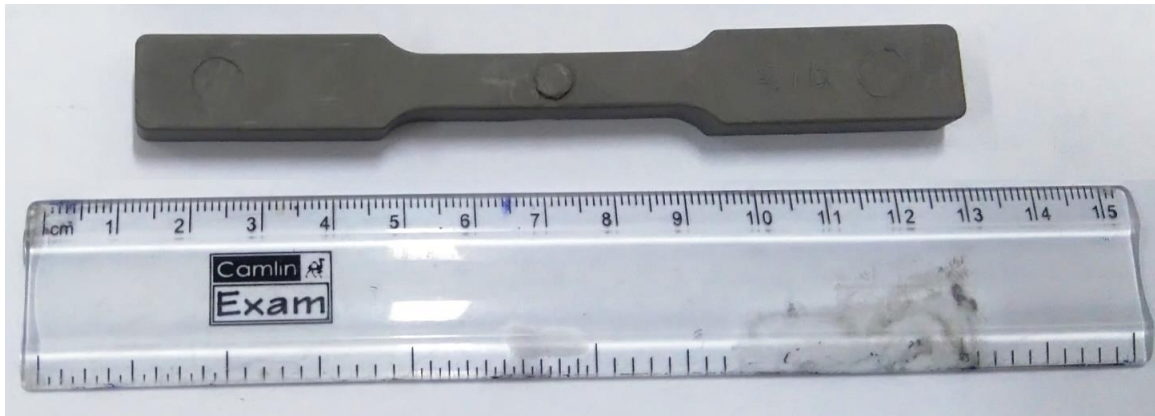
Figure 3.24 Photograph of thermal debound specimen
