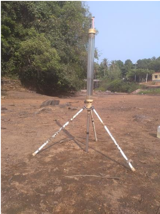
GUELPH Permeameter installed for measurement of hydraulic conductivity of streambed
