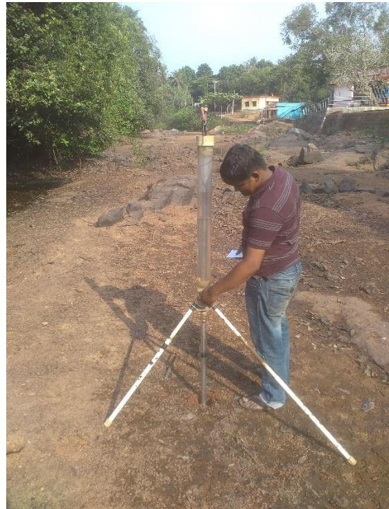
Setting the reservoir knob of GUELPH permeameter
