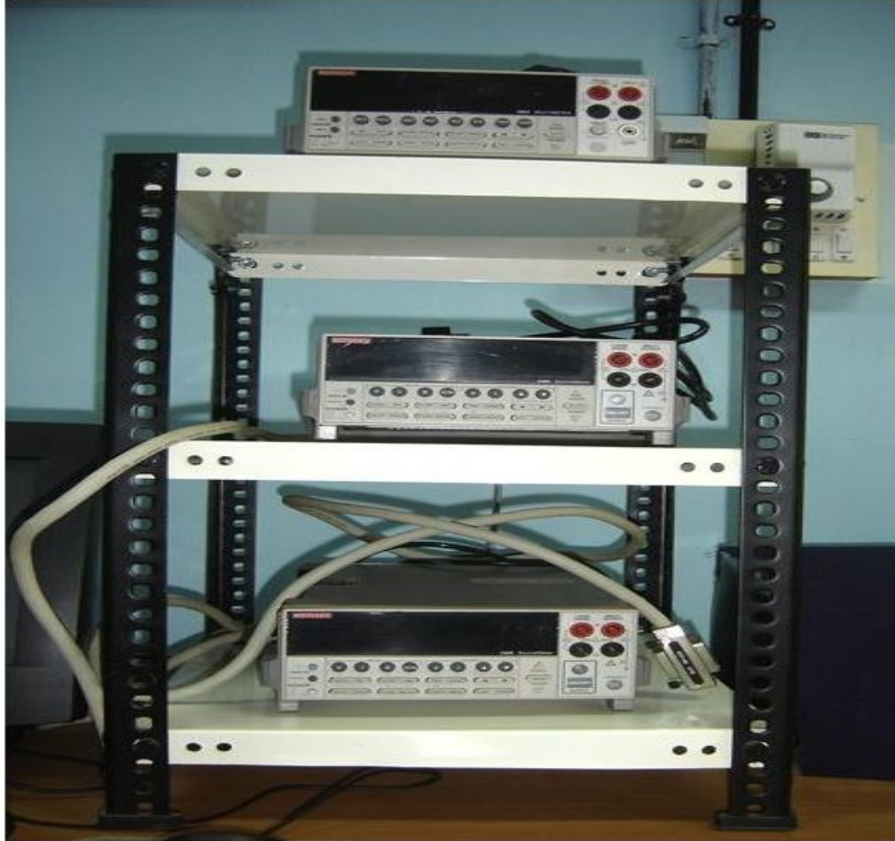
Figure 2.11: Keithley Multimeter (2000) and Keithley Sourcemeters (2400) used in the present study
