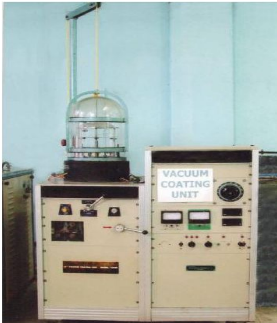
Figure 2.2: Vacuum coating unit (HIND HIVAC 12A4D) used in the present work
