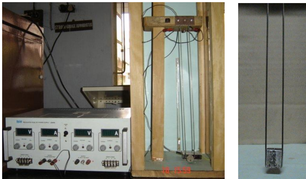
Fig 8.6 Experimental setup of U-tube cantilever beam with tip mass.
