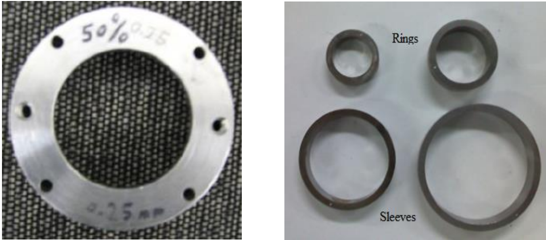
Figure 2.5 Eccentric Sleeve and rings used for creation of eccentricity [Nandi et al. 2009]
