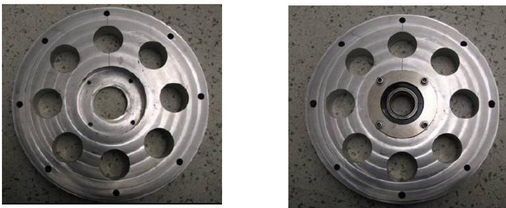
Figure 2.4 End bell and end bell with eccentric sleeve inserted [Nandi et al. 2009]
