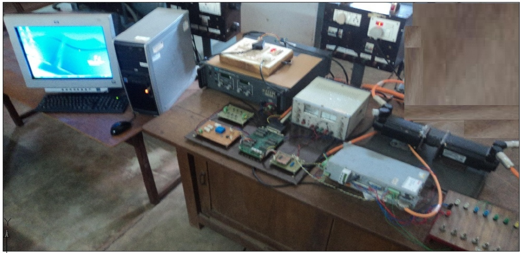
Figure Error! No text of specified style in document..102 Laboratory setup of wave Turbine Emulator
