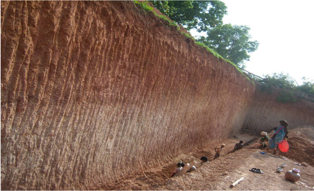
Fig. 4.1a Soil Profile Showing Laterite Layer at The Top, and Partially Shedi Soil Layers to the Bottom of a Highway Underpass, at NITK Campus, Mangalore
