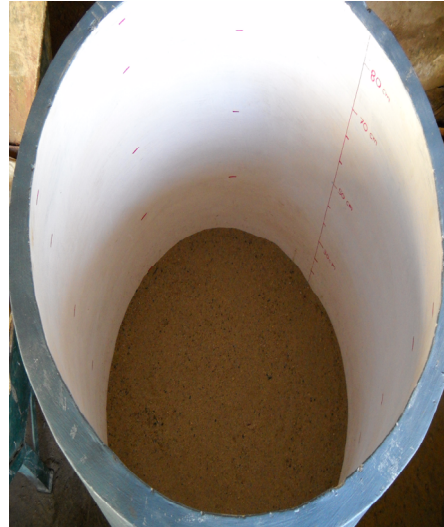
Fig 4.7b Mould Filled with 10cm Thick Sand Layer and Compacted
