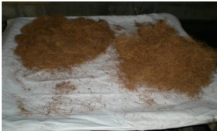
Fig.4.3 Coir Fiber for Reinforcement of Sand and Various Soil Blends
