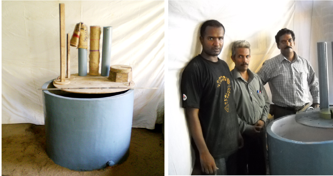
Fig. 4.8a Ferro-cement Test Mould with Accessories for Accelerated Consolidation
