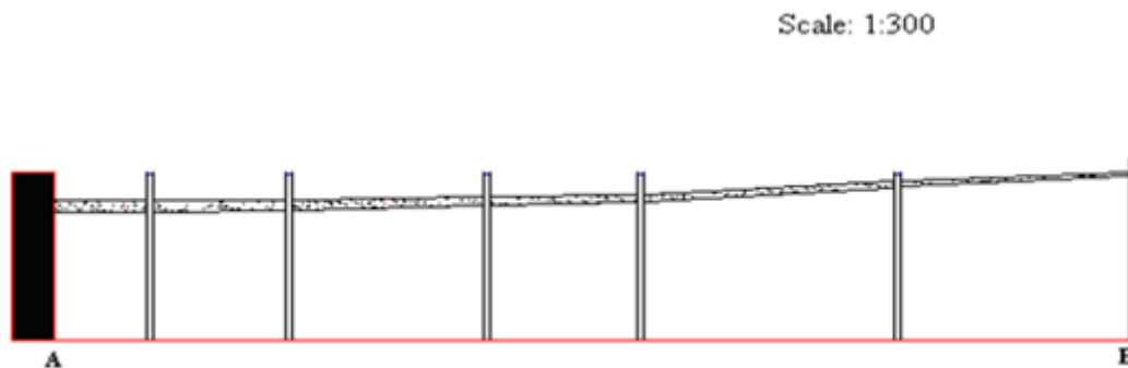
Fig. 9.3 Pattern of silt deposition in the tank area along the chosen section
