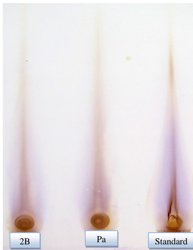
Fig. 4.46 TLC analysis of proteins in surfactant produced by Pseudomonas sp. 2B and Pseudomonas aeruginosa
