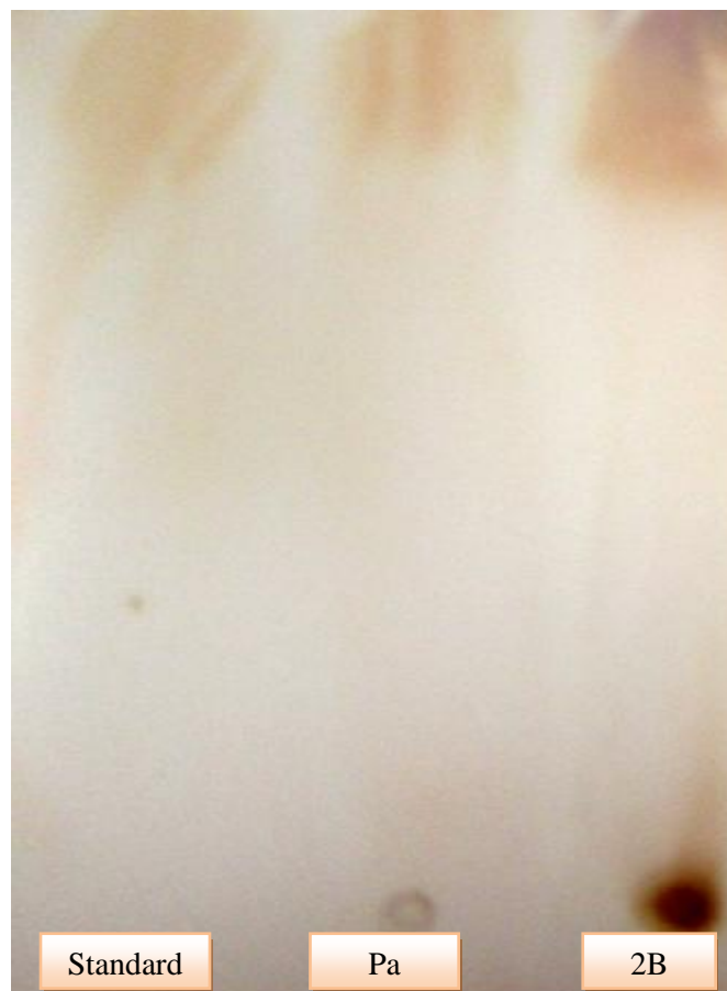
Fig. 4.47 TLC analysis of carbohydrates in surfactant produced by Pseudomonas sp. 2B and Pseudomonas aeruginosa
