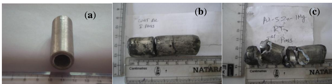
Fig. 5.5 Tubular specimens (a) Cast Al before ECAP (b) Cast aluminium (c) Al-5Zn-1Mg after first pass
