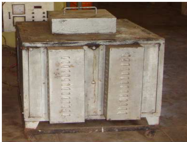
Fig.3.6 Salt bath furnace for austempering treatment
