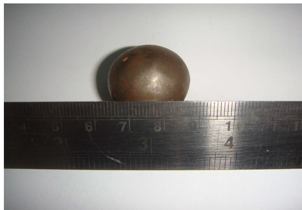
Fig.5.25 Photograph of the ADI balls remains unaffected even after milled for 40 hours in the ball mill
