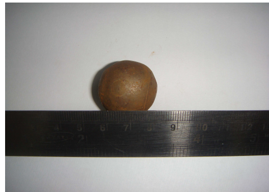
Fig 6 AlCrN coated ADI milled
