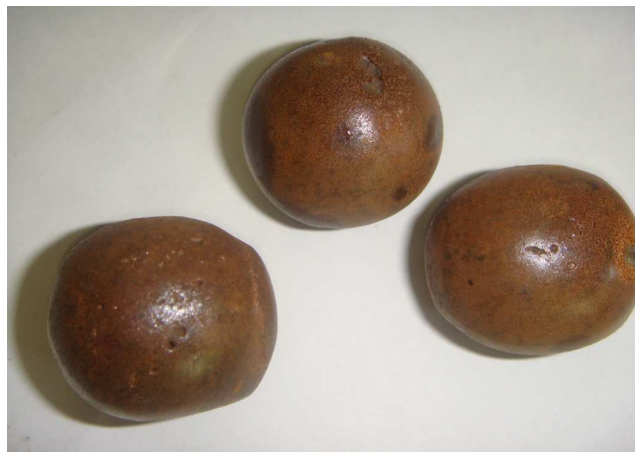
Fig.5.24 Photograph of the milled forged En 31 steel balls reveals damage in the form of porosities on the surface
