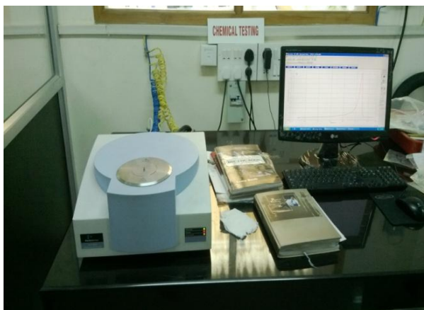
Figure 4.21: Differential Scanning Calorimeter
