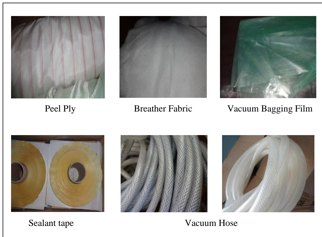
Figure 3.9: Materials for Processing VARTM of Composites
