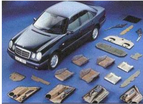
Figure 2.11: Interior components made of reinforced natural fibre composite for E- Class car [Ellision and Naught 2000; Greencarcongress 2008]
