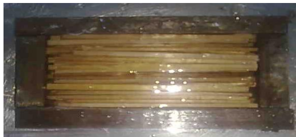
Figure 5.2: Maize Long Fibres with Polymer Matrix in the Mould
