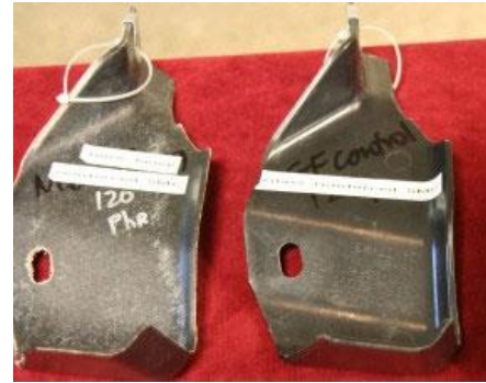
Figure 2.12: Part of hemp and glass plastic bonded with resin solutions for bus seat [Tylor 2002]
