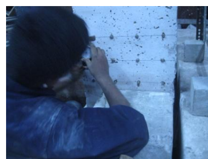
(f) Crack measurement by crack measuring microscope (g) Strain measurements
