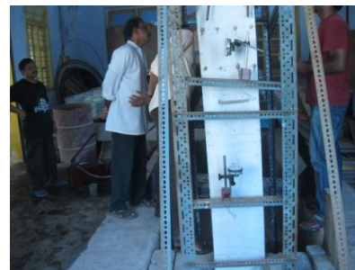
(b) Specimen fitted with dial gauge
