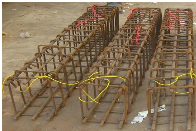
Fig. 3.3 View of reinforcement details of beam specimens
