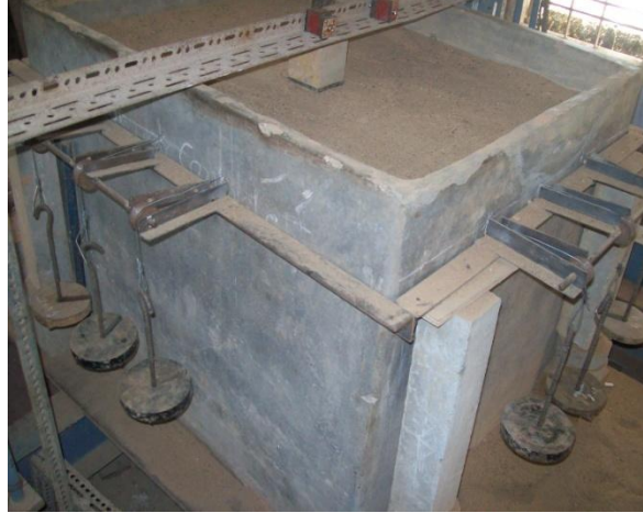
Fig.3.8. Prestressing force applied through three pulleys
