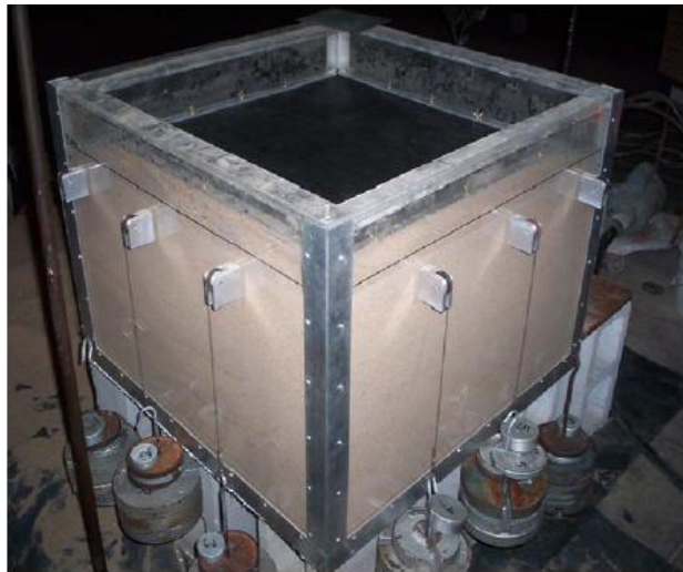
Fig.2.4 Experimental setup for prestressing the geotextile (Lovisa et al., 2010)
