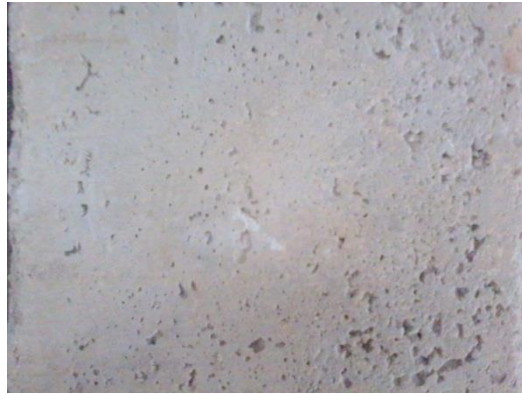
Fig. 6.2 Surface of VC mortar exposed to 600°C
