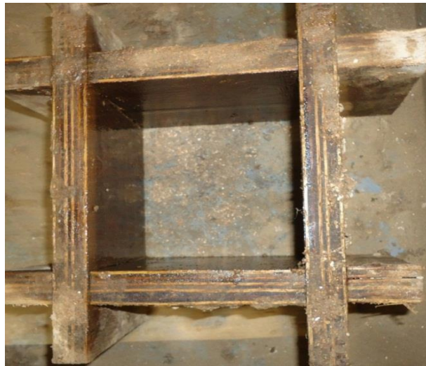
Fig. 3.5 Mould of size 120mm x 120mm x 120mm
