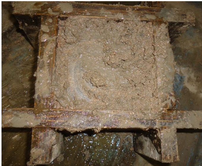
Fig. 3.7 Application of plaster to the concrete cube
