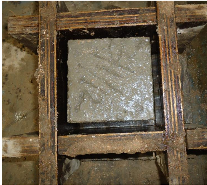
Fig. 3.6 Cube placed in the mould
