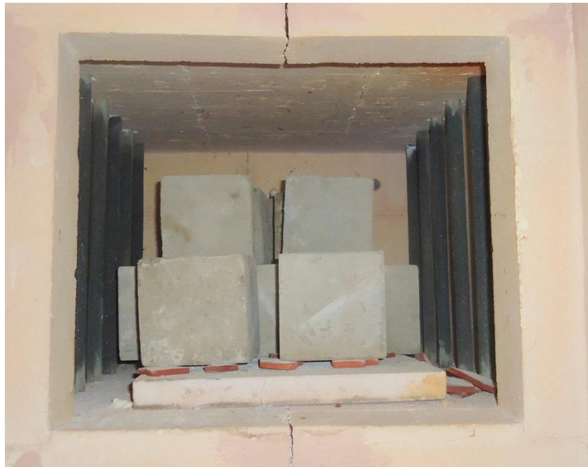
Fig. 3.4 Arrangement of 15 cubes inside the furnace-2
