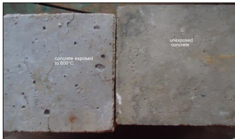
Fig.4.1 Surface of concrete exposed to 800°C
