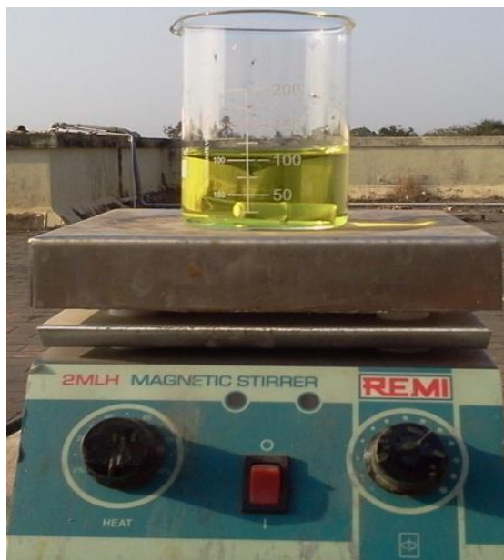
Figure 3.5 Photographic image of the batch stirred reactor experimental set-up for solar photocatalysis.
