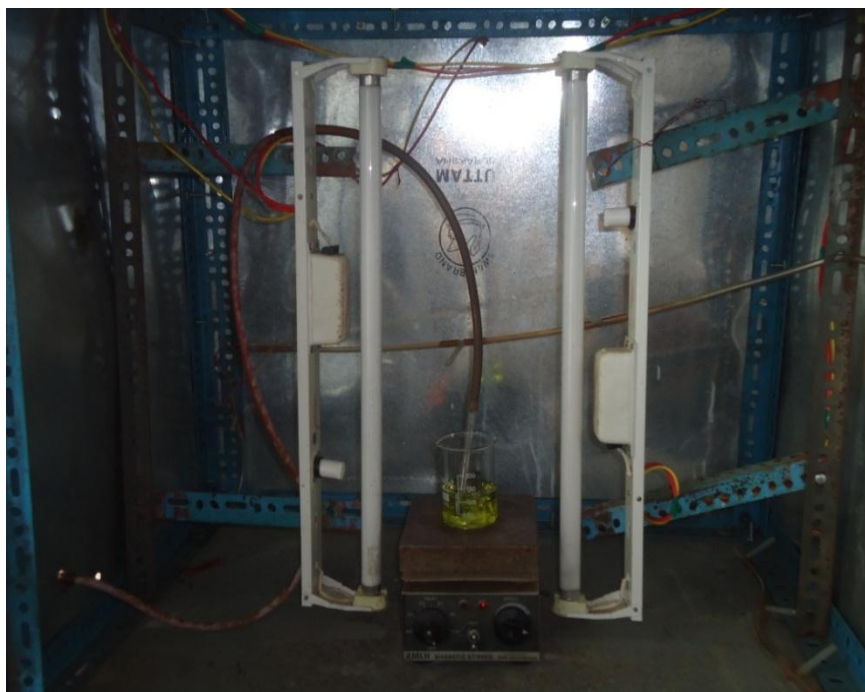
Figure 3.3 Photographic image of the batch stirred reactor experimental set-up for UV photocatalysis.
