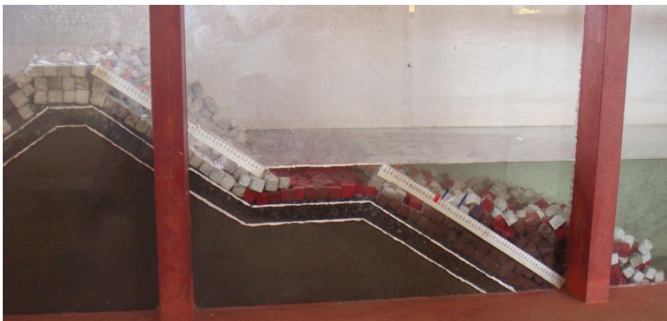
Plate 3.9 Reshaped profile of berm breakwater after storm duration
