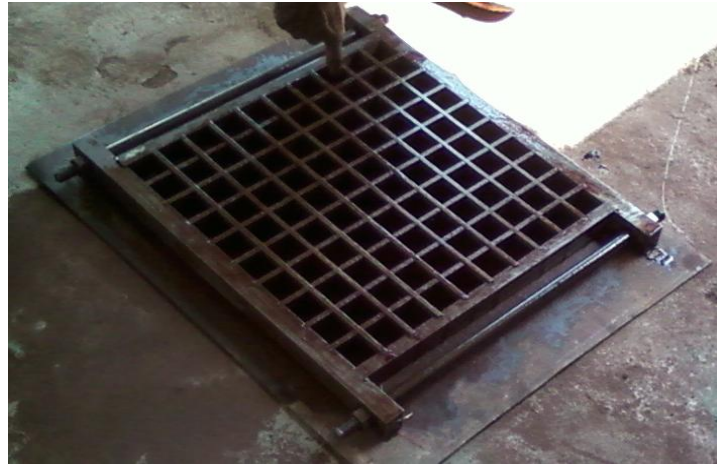
Plate 3.2 Mould for cube casting
