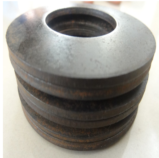
Fig. II.8. (a) Schematic and (b) photograph of series arrangement of Belleville springs.
