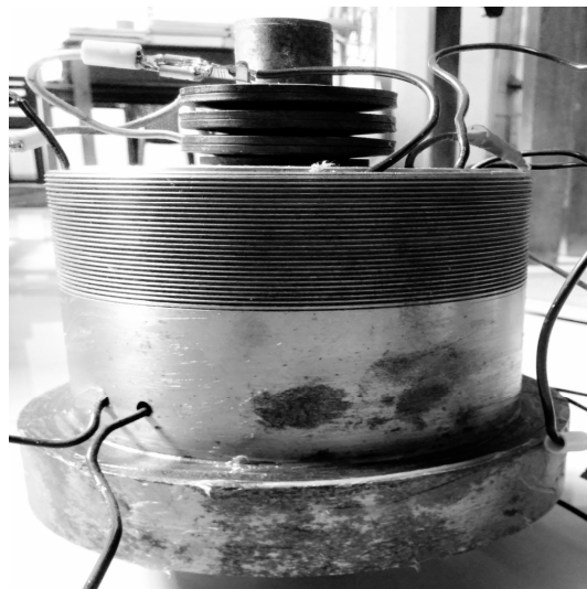
Fig. IV.4. Actuator housing with coaxial coils, end plunger and Belleville springs.
