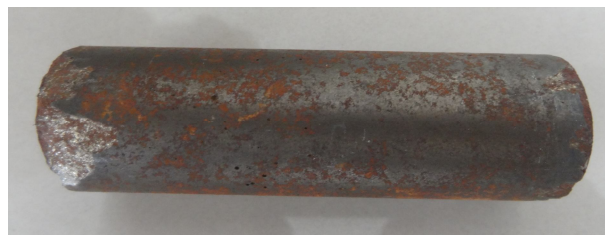
Fig. II.1. Magnetostrictive material (Terfenol-D) test specimen (DMRL, Hyderabad).
