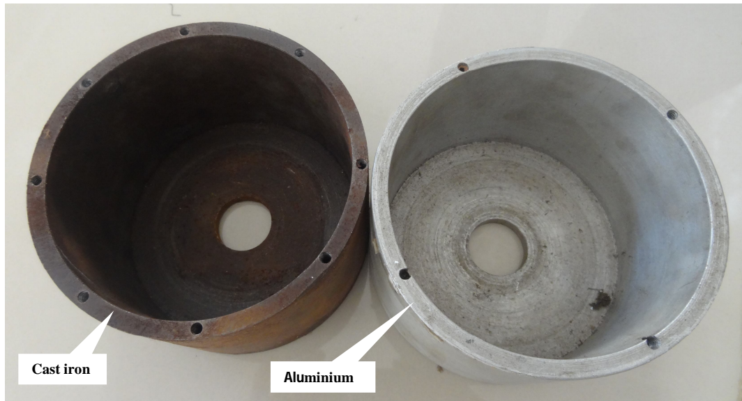
Fig. II.3. Housing materials (cast iron and aluminium) used to test the performance of a Terfenol-D actuator in the experimental setup.
