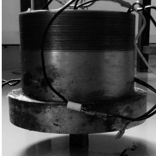
Fig. IV.3. Actuator housing with coaxial coils.
