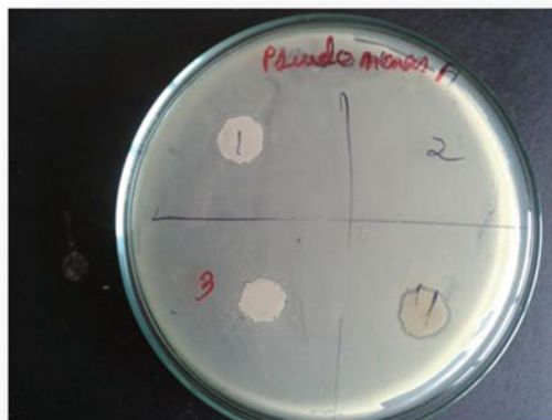
Fig. 7 Antibacterial inhibition zones by TUAgnps impregnated cotton bandage gauze against Pseudomonas aeruginosa
